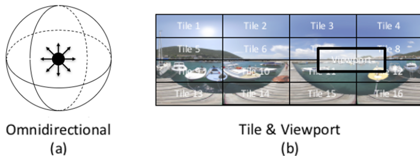
Figure 1: (a) Users watch 360° videos by moving their viewport to point to any direction in the enclosing sphere (b) each frame of the 360° video is broken up into tile frames [5].
